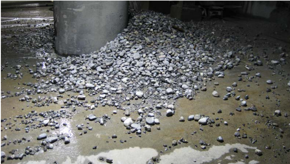
Figure 2 – Rock flushed from a rougher row after a significant rock event
